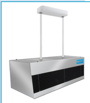
Figure 2 – Shows the top of Hygeaire® Model LIND24-EVO-2PM (above). Note the two mounting holes on the top of this fixture (these are for the Pendant Mount Canopy Set attachment). The fixture is to be mounted at a minimum height of 7 feet from the bottom of the fixture to the floor, in a location that must be able to safely support 32 pounds.
